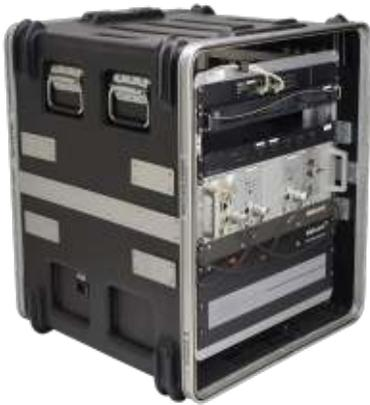
The ET-1 case supports Zetron's standard 19" subrack and has an internal mounting height of 6, 9, 12 or 15 RU. The case is weatherproof and constructed from high-density polyethylene with reinforced walls. It has recessed handles, smooth latches, anodized valances and a pressure relief valve. The rack is shock mounted and the lid gasket is watertight. Racks can be mounted inside the front and back of the case.
