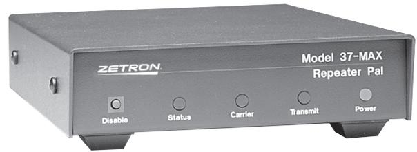
The unit recognizes when a subscriber unkeys with reverse burst or DCS turnoff code, silently muting repeater receiver audio to prevent squelch tails. This ensures that listening radios are quieted instantly without an annoying noise burst.
