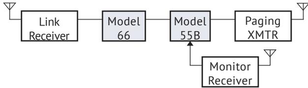
Analog pages stored as audio directly from a receiver monitoring the paging channel.
