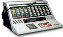
The Model 4018 supports a total of 76 buttons for control of system, channel, auxiliary I/O, and paging functions.
